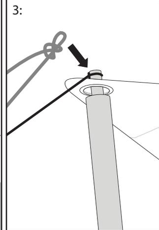
1: Place the Support Pole through the eyelet in the Insert.
