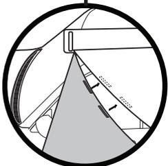
2: As the Front Edge Zippered Insert is being attached to the Batwing, fix the velcro tabs to the awning along the length of the inserts zipper.
